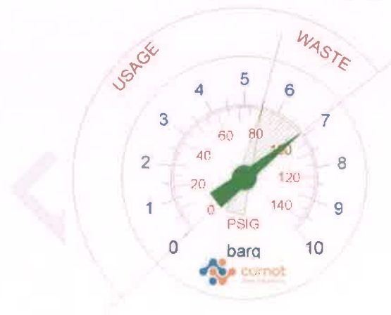
Figure 4. Artificial Demand of Air Compressor
